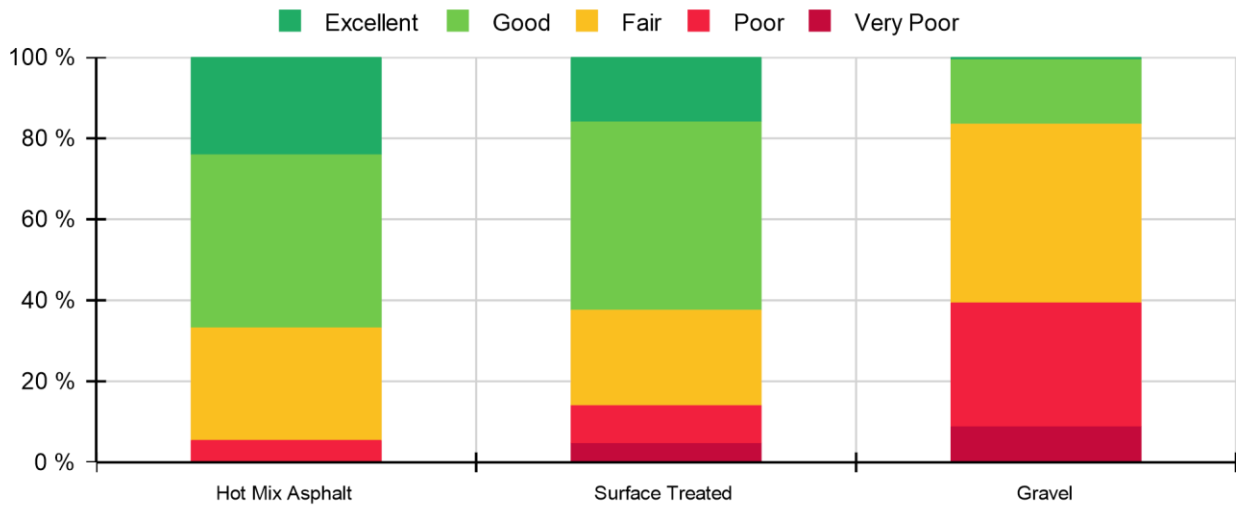
Figure 2: Surface Type Condition Status
