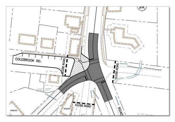
Recommendations have included closing off multiple roads and the addition of a signalized intersection (see Figure 2).
