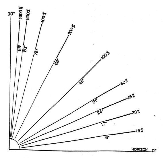
Expressing slope as a percentage permits easy comparison of the relationship of the vertical (rise) to the horizontal (run). For example, a 30% slope will rise 30 m vertically over a horizontal distance of 100 m.
